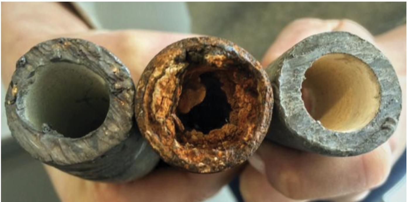
EXAMPLES (FROM LEFT) OF A LEAD PIPE, A CORRODED STEEL PIPE, AND A LEAD PIPE TREATED WITH PROTECTIVE ORTHOPHOSPHATE
